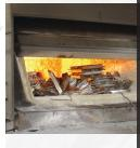
Our special dry out and heat up technology is based on the use of Hotwork International High Velocity Burners operating on an excess air basis, which have been especially developed for the dry out and heat up of all types and sizes of furnaces/kiln/vessels and refractory lined components. The system permits a positive pressure assuring uniform temperatures in the vessel/piping components etc.
